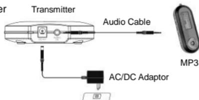
Connect the barrel end of AC/DC adaptor to the DC input of the back panel of DAS-110, AC end to your AC outlet
